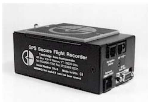
Secure flight GPS flight recorders are carried by every competitor and track the flight creating a digital file called a flight trace which is used for scoring. Image from Cambridge Aero Instruments.
